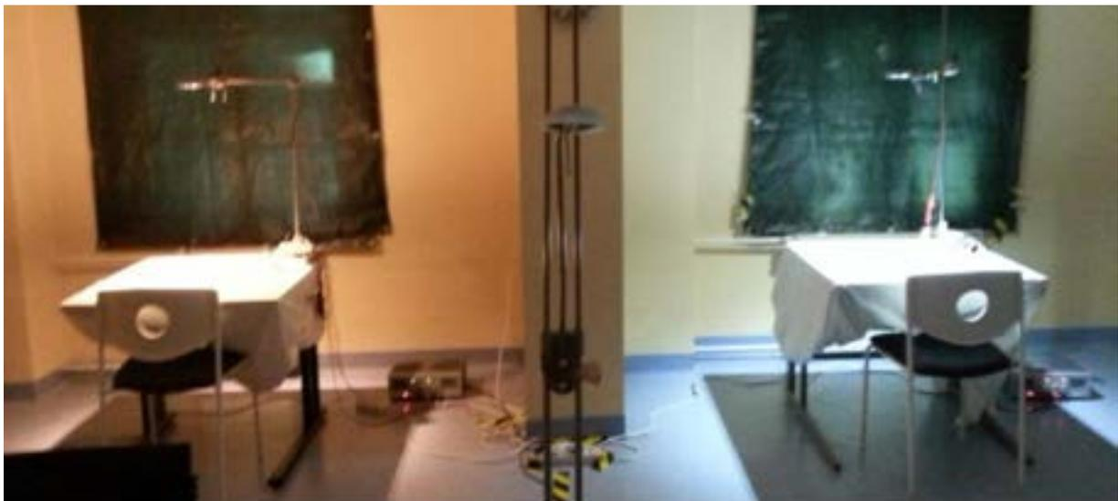
*Figure 2 shows a representative example of the lighting situation with the warm white LUCTRA TABLE PRO desk lamp (on the left) and on the right the situation with the cold white LUCTRA TABLE PRO desk lamp, as tested during the study.*
