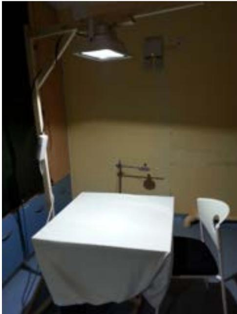
*Figure 3: shows the lighting situation for the bright light (BL) reference illumination with an LED spotlight placed above the desk.*
